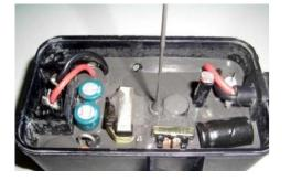
Flextein<sup>™</sup> SEA2015 is a two-component thermally conductive RTV silicone sealant for insulating and protecting electrical and electronic components from application and environmental stresses. This rubber like compound resists to shock and vibration, and for exclusion of moisture and corrosive agents. High conductivity makes Flextein<sup>™</sup> SEA2010 suitable for electronic components or packaging requiring heat dissipation while sealed.
